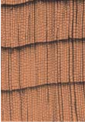
Cross-section of western red cedar showing the narrow latewood
